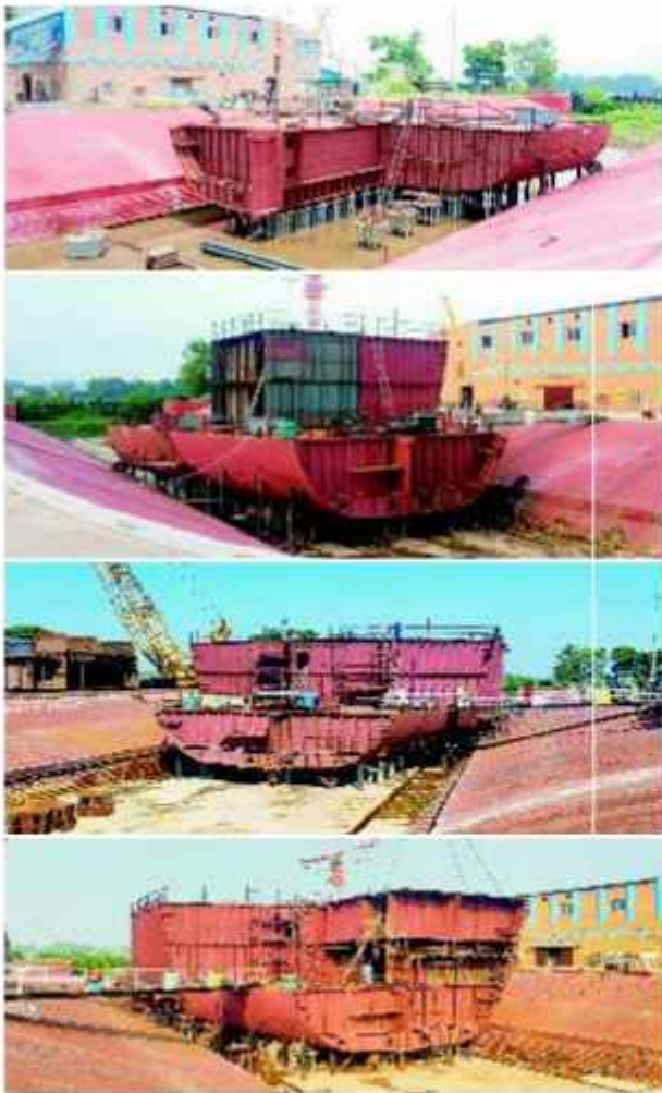
Fig. 3.10: Sequential stages of vessel block assembly at GRSE dry dock, Kolkata.
