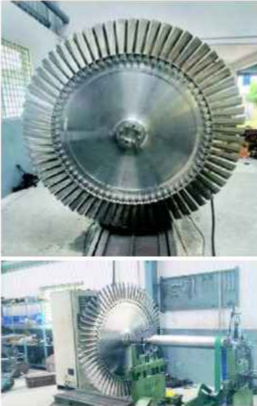
Fig. 2.1.8: Dynamic balancing of the open cycle OTEC turbine rotor at Kavaratti, Lakshadweep.
