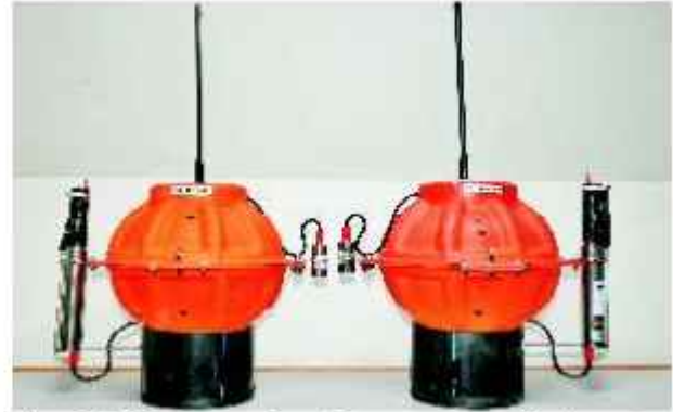
Fig. 2.1.11: Deep Sea Autonomous Underwater Profiling Float (DAUPD - 2000/4000 m).
