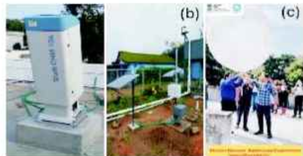
Fig. 4.7: Instrumentation at NCESS atmospheric observatories: (a) Ceilometer installed on the rooftop of the NCESS campus, (b) Laser Precipitation Monitor at the High Altitude Cloud Physics Observatory in Munnar, and (c) Radiosonde launch at the NCESS campus.
