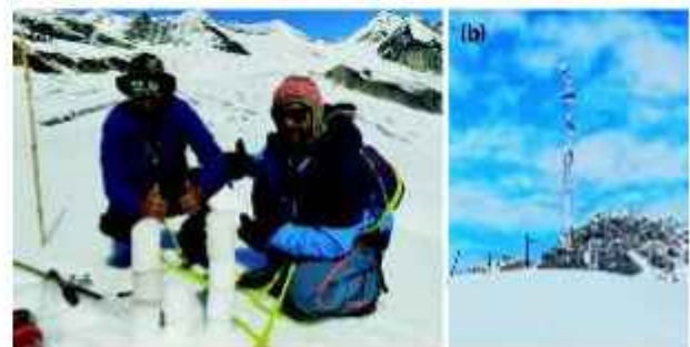
Fig. 2.2.17: (a) Snow core sampling from the accumulation zone of Samudra Tapu glacier for snow density measurement and total annual snow accumulation, and (b) AWS near Himansh station with snow-covered surface.
