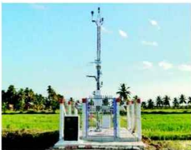
Fig. 4.5: Scintillometer facility established by NCESS at the Tamil Nadu Rice Research Institute (TRRI), Aduthurai Critical Zone Observatory.
