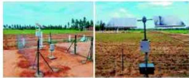
Fig. 4.6: Soil moisture profiler installed at the NCESS Critical Zone Observatory in Aduthurai.
