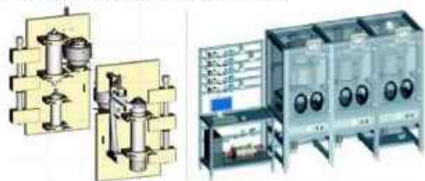
Fig. 3.8: Design of the high pressure retainable water sampler (left) and the high pressure microbial culture system (right).
