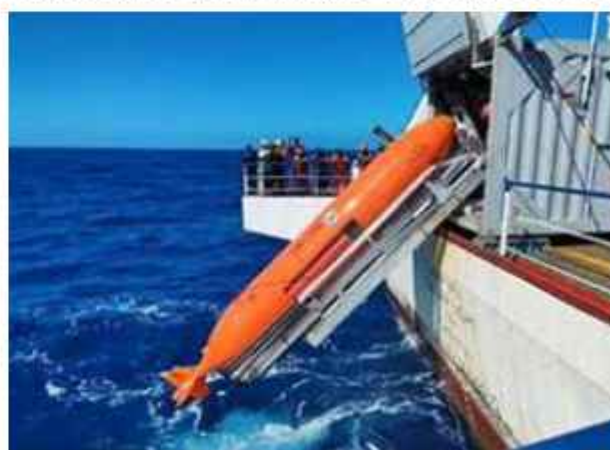
Fig. 3.9: Deployment of the AUV from ORV Sagar Nidhi for hydrothermal vent exploration.
