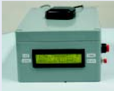
Handheld GPS with in-built memory
