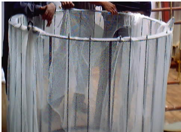
Experimental cage developed for in situ TS measurements
