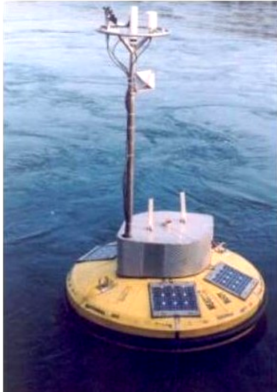
A fully indigenised data buoy with INSAT communication for data transmission deployed off Ennore Port on 31 st December 2002
