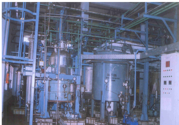
Bulk sulphide precipitation and dissolution section of pilot metallurgy plant at HZL
