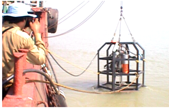
In-situ soil testing equipment being launched at Haldia
