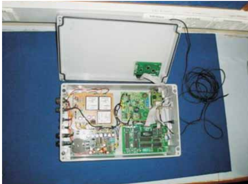
200 kHz integrated Echo-Sounder developed and successfully tested
