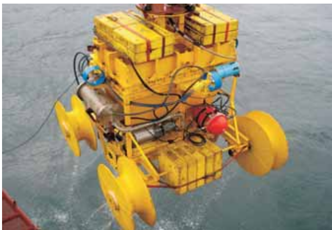
Subsea Artificial Nodule Laying System being launched
