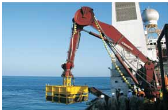
Crawler dummy weight launched through LARS from ORV Sagar Kanya
