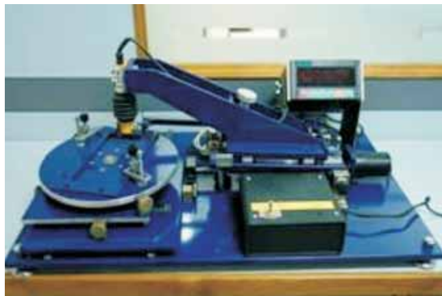
Barnacle adhesion tester jointly developed by UCTM (Bulgaria) and NIOT (India)
