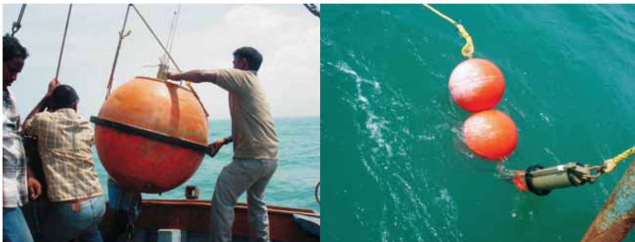
Wave rider buoy and current meter deployed in the Bay of Bengal
