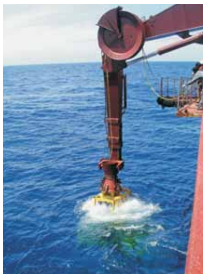
Soil tester entering splash zone
