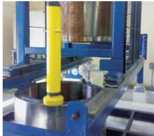
Testing of Argo Float Main components of Hyperbaric Test Facility
