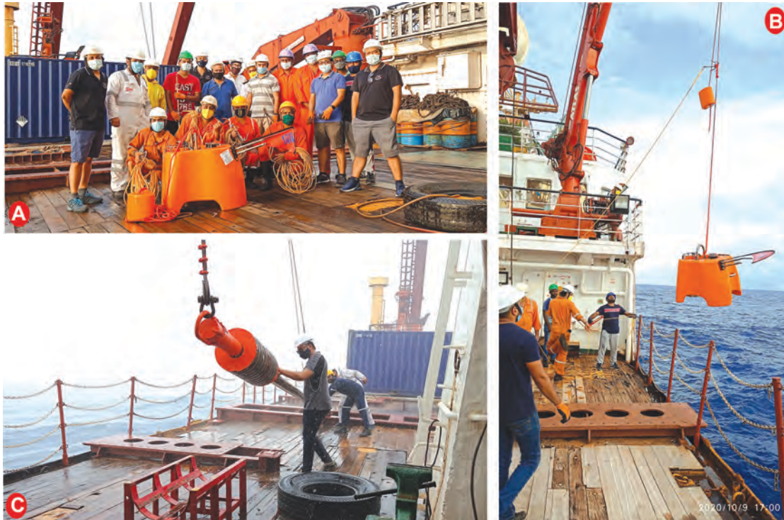
Fig. 5.6 (A) OBS recovery team during the SK-368 cruise onboard ORV Sagar Kanya, (B) SK-368 team retrieving an OBS system and (C) Gravity coring operation
