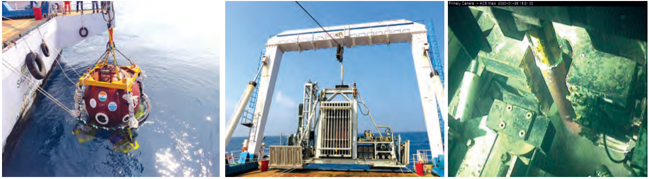
Fig. 3.19 (a) Shallow water personnel sphere deployment and testing onboard Sagar Nidhi (b) Deployment of Autonomous Coring System at Gas Hydrate Site in Krishna Godavari Basin (c) Subsea operation at 1070 m
