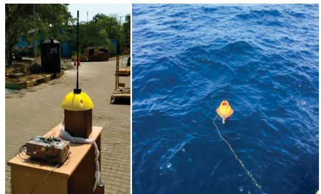
Fig.3.20 DAUPD - RF Antenna test & Field trials.
