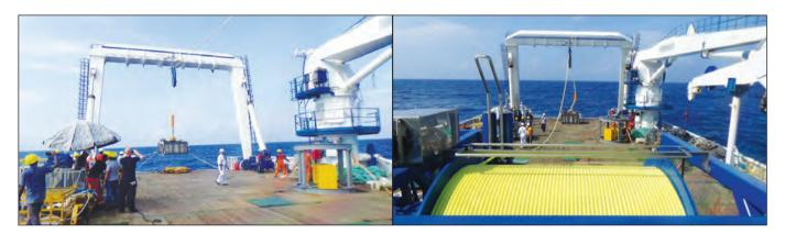
Fig. 3.11 Winch and Umbilical cable test on-board ORV Sagar Nidhi
