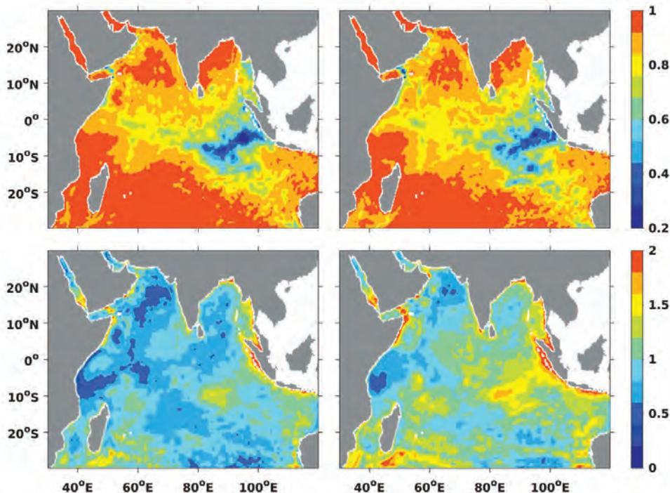
Fig. 3.5 Maps of correlation (top) and root mean squared error (bottom) between AVHRR SST and SST of RAIN (left) and free model (right)
