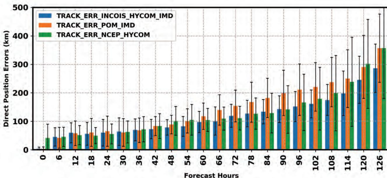
Fig. 3.4 Comparison of mean direct position errors at different forecast lead times from HWRF coupled to HYCOM, POM and of NCEP run.
