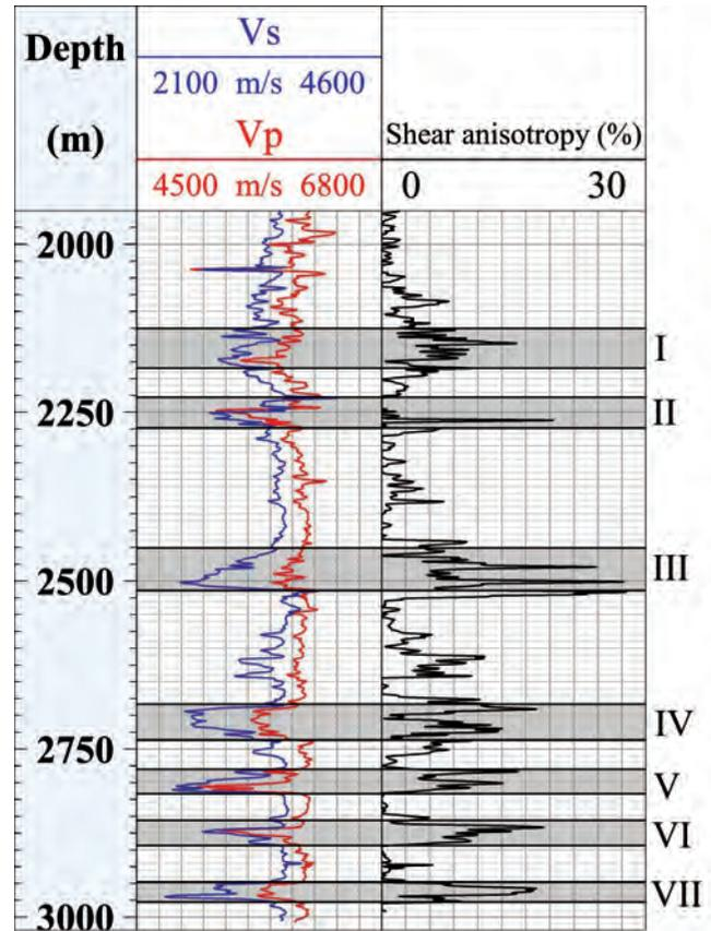
**Fig. 5.4** Depth profile of Vp, Vs, and shear wave anisotropy computed from cross-dipole sonic logs in the basement section 2,000–3,000 m in the Koyna Pilot Borehole. Zones of anomalous physical and mechanical properties are numbered I through VII (grey shading).
