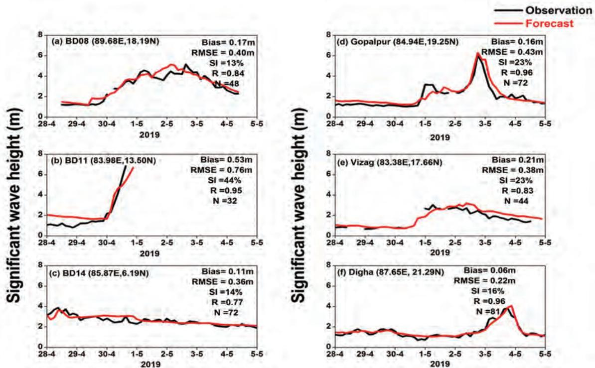
Fig. 3.1 Significant Wave Height forecasts issued by INCOIS are compared with buoy data at various locations during the passage of Fani.
