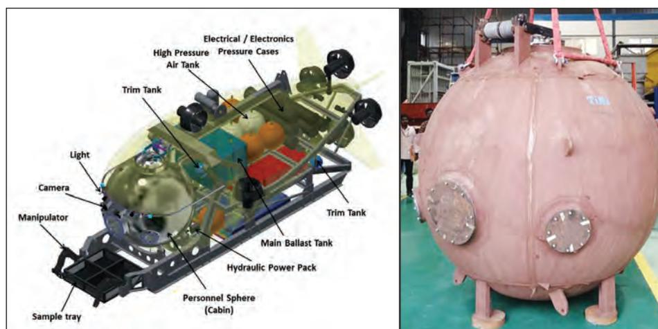
Fig. 3.10 Schematic of manned submersible and Shallow water spherical hull
