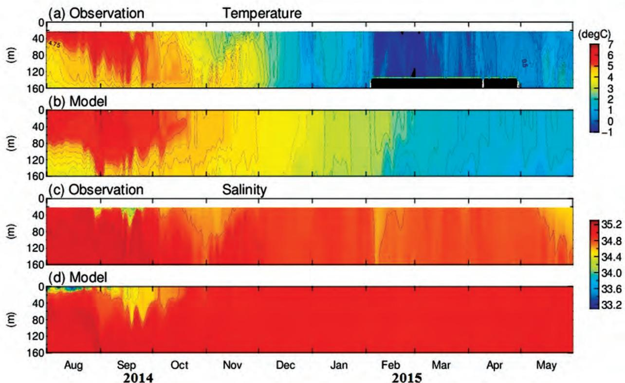
Fig. 4.7 Evolution of temperature and salinity from observations and simulations during 2014-2015. Upper 25 m data is not available in observations.
