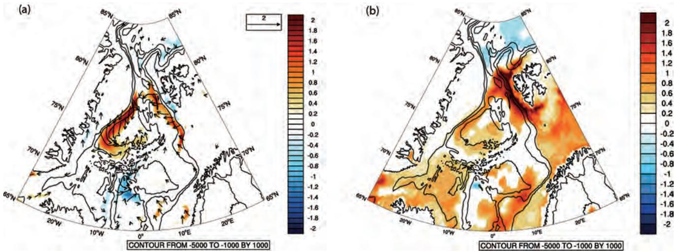
Fig. 4.5 (a) Regression of 700m depth integrated flow speed anomaly ( $\text{cm s}^{-1}$ ) on AW temperature in the Fram Strait. The shading indicates the magnitude of the of the flow speed. (b) Regression of 700m depth averaged ocean heat content ( $109 \text{ J m}^{-2}$ ) relative to  $2 \text{ }^\circ\text{C}$  on AW temperature in the Fram Strait. Only regression coefficients significant to 99% confidence level are shown.
