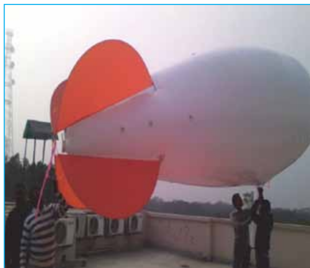
Fig. 2.2: Tether Sonde Balloon Observations upto 1000 m were taken during 3 to 23 January, 2016.
