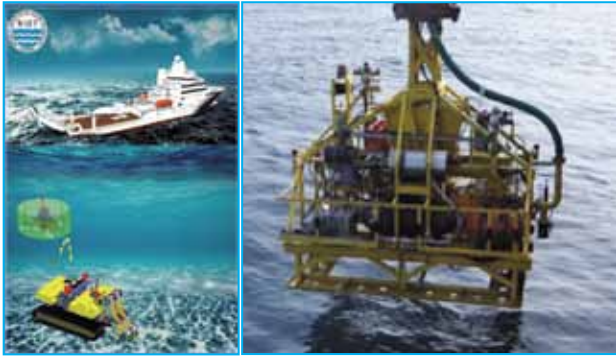
Fig 3.15: Schematic of the Integrated Mining System & Skid for testing positive displacement pump
