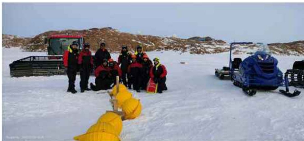
Figure 4.9. Deployment of ice-tethered mooring near Bharati Station (69°24'S, 76°12'E), Prydz Bay in July 2023. This mooring system will measure temperature, salinity and ocean currents in a water column of 120 m depth during the austral winter.
