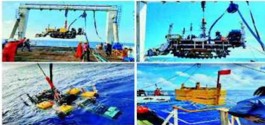
Fig 7.1c : Deployment and testing of mining system in Bay of Bengal at 3300 m at the Central Indian Ocean during Mar-Apr 2023 and deployment of deep sea mooring at PMN site
