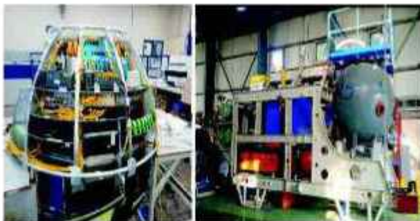
Fig 7.1b : Progress in the development of personnel sphere with VSSC-ISRO and Fig 1c Assembly of mansub internal electronics assembly and mock up frame with assembled components.
