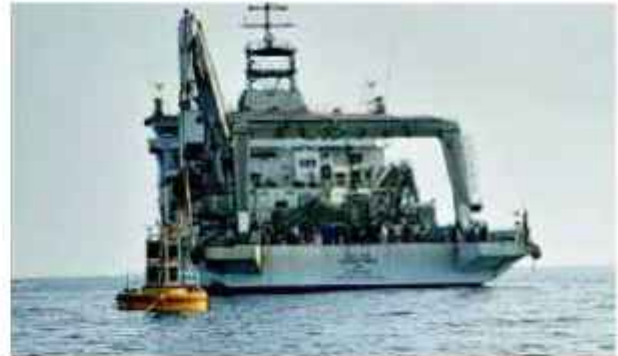
Fig 7.5b : Deployment of buoy system using Sagar Nidhi.
