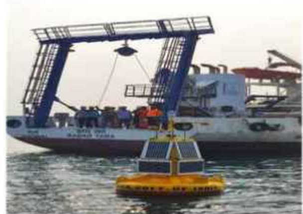
Fig. 3.12 Automated sensor-based water quality buoy at Chennai.
