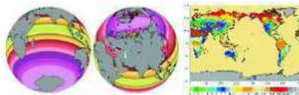
Fig. 2.23 The new ocean grid developed for IITM-ESM (left panel) and land-use land-cover data based on NRSC over Indian region with 24-type vegetation types implemented in IITM-ESM (right panel).
